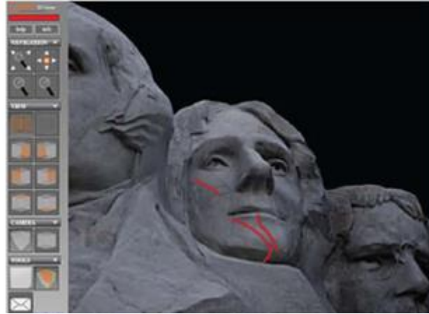
Image showing CyArk's 3D viewer being used to manipulate a 3D model of Mt. Rushmore and identify cracks in the monument
